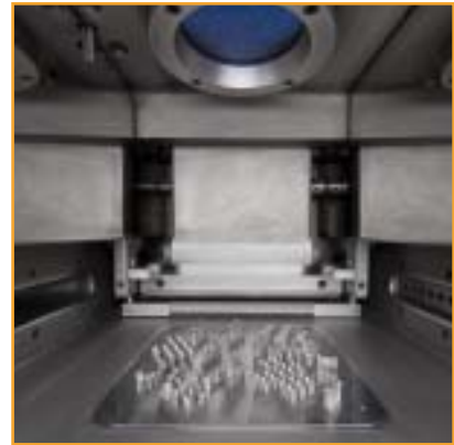
Laser melting machine build chamber
